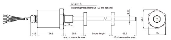
Note: It is equipped with standard Magnet ring kit 288501, with magnetic isolation gasket and fixing screw.
